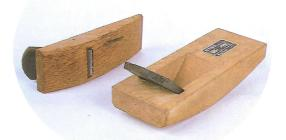
To plane the base of the trunk a carpenter's plane is used like the ones in the photograph at the left.
